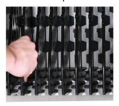
6. Slide retaining metal strip into place & replace thumbscrew.
