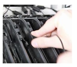
5. Use the supplied Cable Clips to fasten each cable to the divider by pressing down firmly, securing the cable in place.
