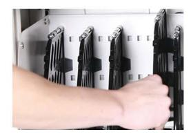
2. If your device is thicker than 1", locate & remove thumbscrew by turning counter clockwise.
