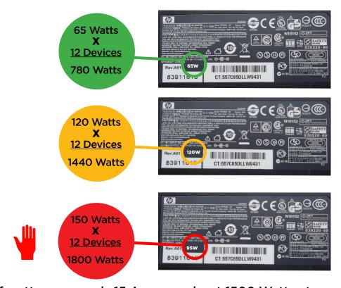
If wattage exceeds 15 Amps or about 1500 Watts at one time, you may trip a circuit breaker; Remove devices accordingly.
