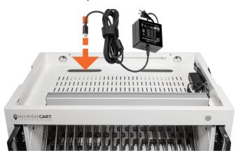
Remove Top Panel by pressing the Latches at the same time, then lift up.
