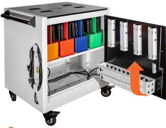
4 Loosen thumbscrews, then pull up & forward to remove. Place 4 device (DC) power cords into each Guide. Re-mount Guide to door and tighten the thumbscrews.
