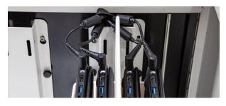
Open a side door and locate the AC Adapter Basket. For iPads or tablets, lift it off the door, flip the basket so that the power strips are facing upward.
