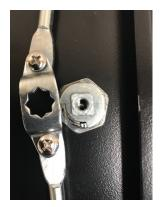
Starting with the back of the door and the center screw removed from the lock assembly, the cam, rods and back of lock assembly should look like this.
