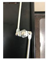
Turn the key 90 degrees to the unlocked position and check that the rods are flush or slightly recessed into the door to allow it open.
